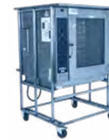
397 Steam oven 380 V / 32A + neutral 16 kW - P 17 connection. Independent water tank, capacity 3 L. Heat range from 50 to 270°C. Supplied with 10 shelves gn 1/1 (53 x 32,5 cm). Space between the shelves : 6 cm. OD : L 96 ; I 108 ; H 165 cm. ID : L 69 ; I 41 ; H 53 cm. 180 Kg
