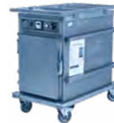
10823 Gastro Fan oven 220 V Electric 220 V / 16A - 3,5 kW. Thermostatic control range from 0 to 300°C. Supplied with 6 shelves gn. OD : L 58 ; I 93 ; H 94 cm. 103 Kg
