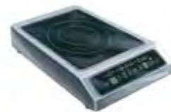
25202 Induction hotplate 230 V - 3 kW Glass vitro top ceramic of 4 mm Double inductor Ø 180 and 280 mm Digital display of the power level and the timer OD : L 39,2 ; P 52,6 ; H 9 cm. 8,5 Kg
