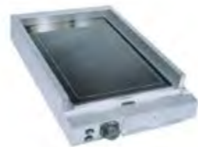
15634 Ceramic flat griddle 220 V - 2,5 kW. L 40 P 65 H 10 cm. 15 Kg Useful surface : 32 x 47,8 cm Ceramic glass cooking surface. Temperature control, quick set up, low consumption.
