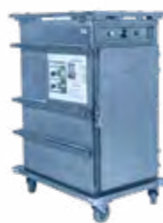
9938 Hot cupboard 8 shelves Electric 220 V / 16A - 3 kW. 1 power supply connection. Max. temperature : 250°C in 60 min. Supplied with 8 pastry shelves 60 x 40 cm. Space between the pastry shelves : 7 cm. OD : L 65 ; I 105 ; H 132 cm. ID : L 40,5 x I 60 x H 85,5 cm 150 Kg
