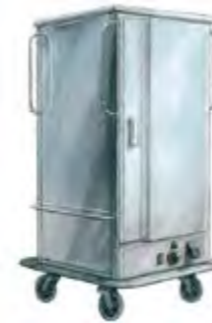
411 Steam turbo fan hot cupboard 8 shelves 220 V / 16A - 2,2 kW. Max. temperature : 150 °C en 50 min. Supplied with 8 shelves gn 2/1 (65 x 53 cm). Space between the shelves : 10,5 cm. OD : L 77 ; I 93 ; H 162 cm. 135 Kg
